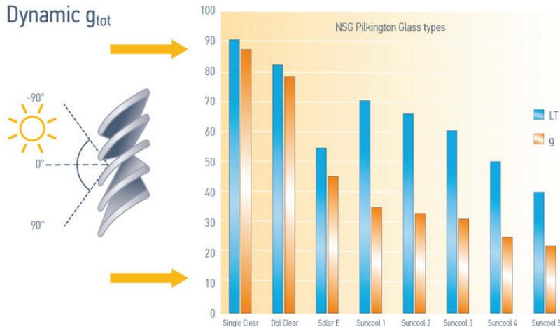
This table shows a selection of glass specifications - from Single Clear, Double Clear and further adding various levels of selective coatings showing the g and LT values (note that buildings today often require a g<sub>tot</sub> around 0,15). Clear glass combined with dynamic solar shading can provide dynamic values.
