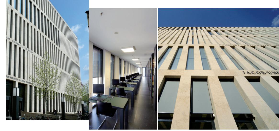
he Jacob und Wilhelm Grimm Zentrum is a building boasting cubist strictness and clarity. The deeply inset window openings have no frames or ledges, while their different sizes ensure architectural diversity. All openings are fitted with automatically-operated sunshades.
